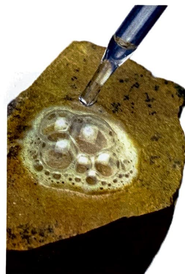
▲ Gas-evolution reactions, such as the reaction of hydrochloric acid (HCl) with limestone ( \text{CaCO}_3 ), typically produce \text{CO}_2 ; bubbling occurs as the gas is released.
